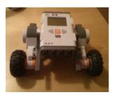
To build and attach the left wheel, follow the previous construction plan but treat it as mirror image. In other words, you want to reverse "left" and "right" to make sure the powered wheel will fit properly on the left side of the brick. Once you attach the left wheel, your robot should look like this (it is almost finished).
