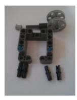
Now add the wheel with the axle to this supporting structure, secure it with the bushing you still have left, and attach the entire structure to the underside of the brick with the motor ports.
