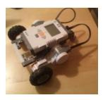
Finally, take a pair of medium or small cables and connect one motor to port A, the other to port C. The finished robot should look something like the picture on the left.
