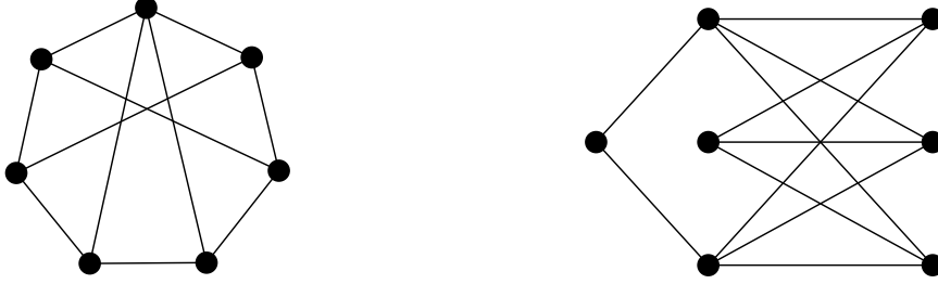
Figure 1: The two maximal graphs of the (7, 11) Tutte polynomial poset. The left graph maximizes all-terminal reliability, and the right graph maximizes acyclic orientations, in the \mathcal{G}_{7,11} graph class. Both parameters may be obtained from the Tutte polynomial.
