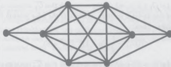
Figure 2: The best 2-edge addition is to introduce a double edge connecting the far left and far right vertices.
